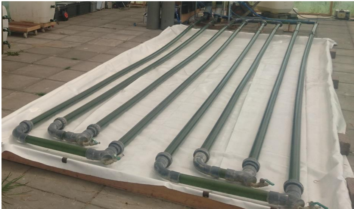
Figure 2 . The tubes of the bioreactor turn green, an indication of vital microalgae. (Source De Wilde and Smits, 2019)
