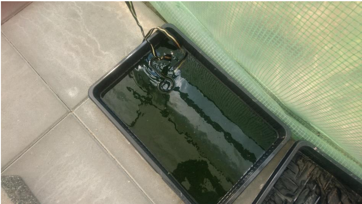
Figure 5 . Harvested microalgae from the wastewater prototype are left to dry (Source De Wilde and Smits, 2019).
