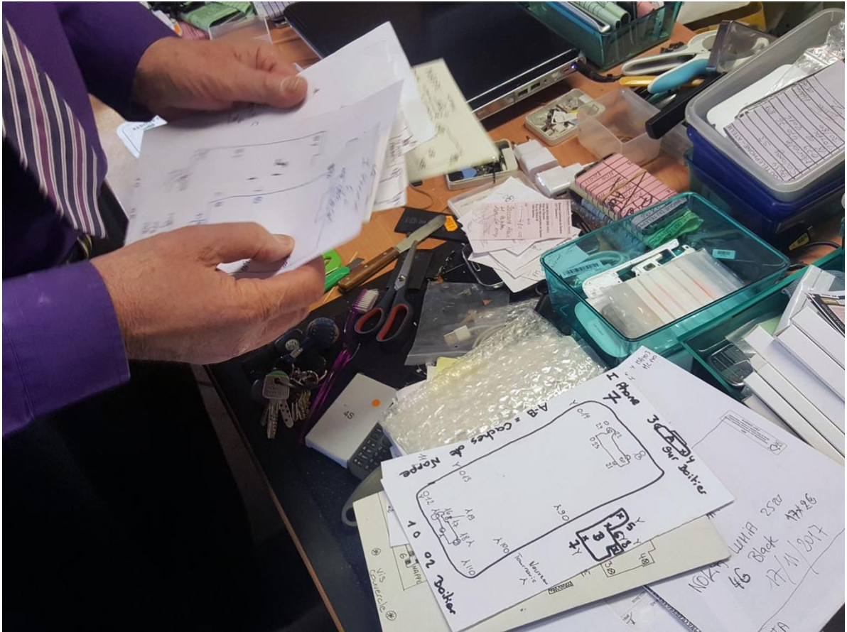
Figure 3 . A series of hand-drawn iPhone 7C schematics reconstituted by a repairer on A5 sheets of paper after disassembling the smartphone. The size of the document corresponds to the actual dimensions of the phone model placed on the sheet of paper, with notes about the location of screws as well as specific connections to the motherboard by ribbon cables. Here again, the annotations are made only for the repairer and mostly focus on how to open the device. (Source Bloch).
