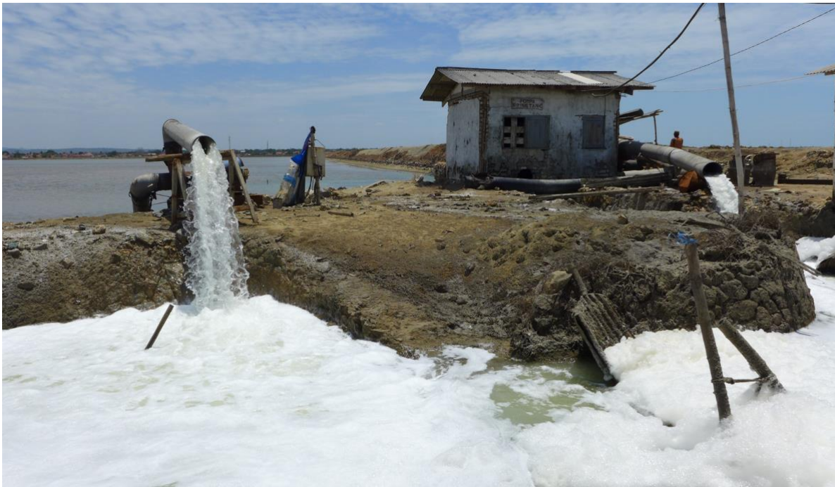
Figure 3. At an industrial scale salt operation in Madura pumps carry brine and bittern between human-made ponds. The liquid bittern, a by-product of salt production, will be released into surrounding waterways. New commercial salt operations in Kupang Bay, Timor are made to emulate the Madurese model, which dates back to the Dutch colonial salt monopoly (Source Author's own).
